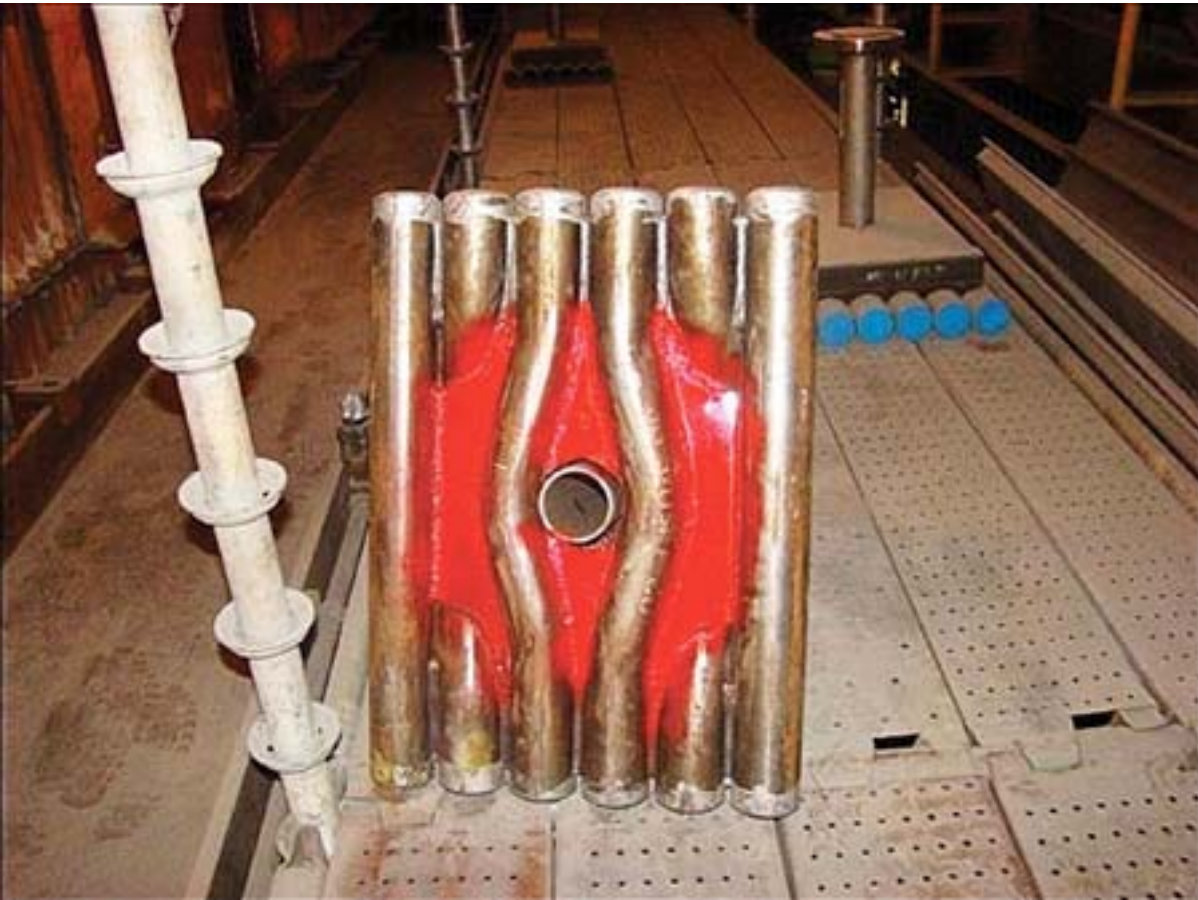
7. Improving the design. The original waterwall penetration had a tendency to slag over, preventing the laser from operating. A new port opening design that minimizes refractory at the opening reduced those problems. Courtesy: Platte River Power Authority
